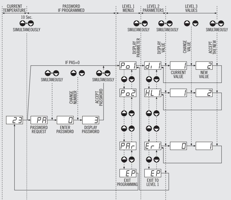
NOTE: If no key is pressed for 25 seconds in either of the previous steps, the controller will automatically return to the CURRENT TEMPERATURE display status without modifying any of the parameter values.
