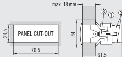
To fix the unit, place the fasteners 1 over the sliders 2 as shown in the figure. Move the fasteners in the direction of the arrow. By pressing tab 3 fasteners may be moved in the opposite direction of the arrow.
